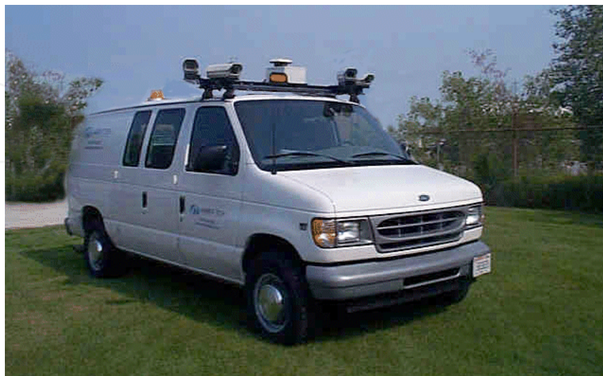
Figure 5. GPSVision™ - with four video cameras achieved by the “LAMBDA TECH INTERNATIONAL” Company (USA) for objectives that are closed to the road arteries
