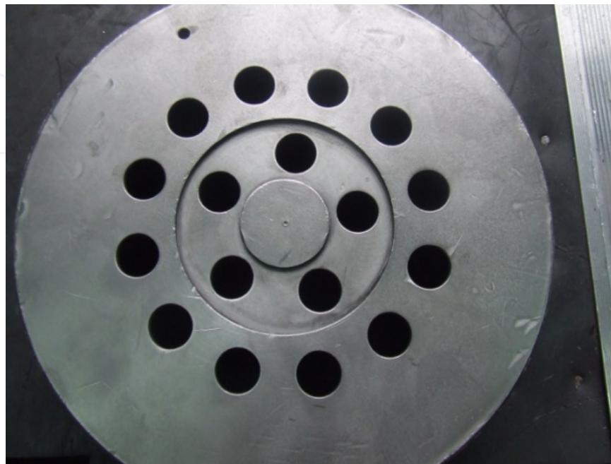
Figure 15. Schematic diagram of 17-hole die with ring-shaped pocket.
