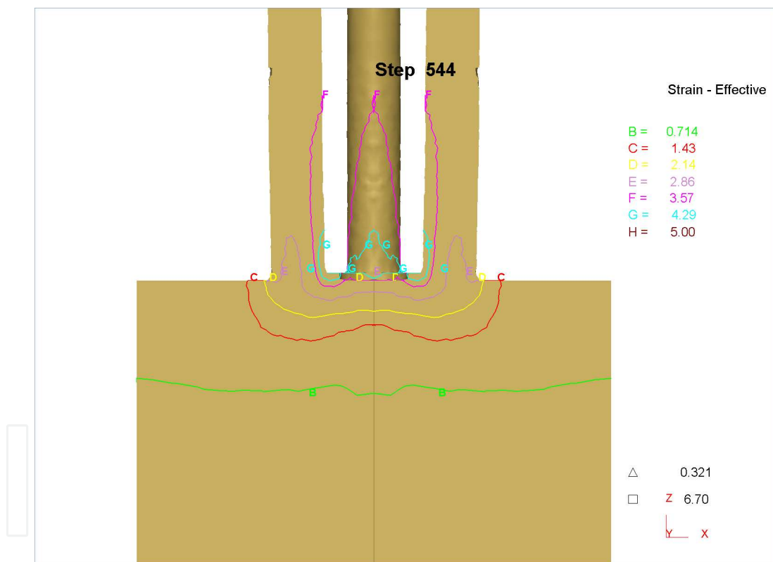
Figure 10. Distribution of intensive strain upon extrusion through ring-shaped pocket die.
