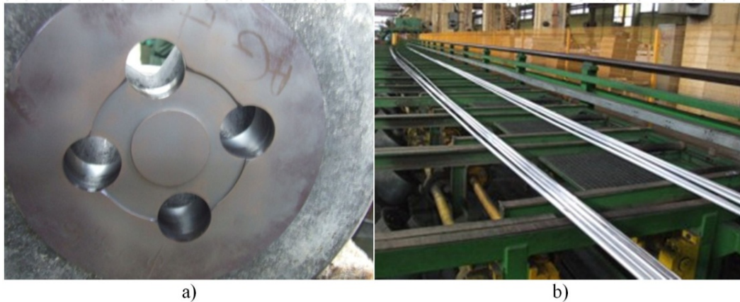
Figure 11. Extrusion tests in industrial conditions through four-hole die, view of ring-shaped pocket die, b) view of extruded bars at press run-out.
