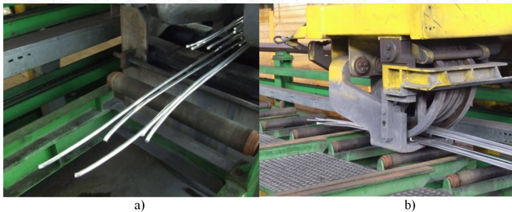
Figure 16. Extrusion of bars through a 17-hole die with ring-shaped pocket, view of bars after exiting the die, b) guiding puller (courtesy of Grupa Kety).
