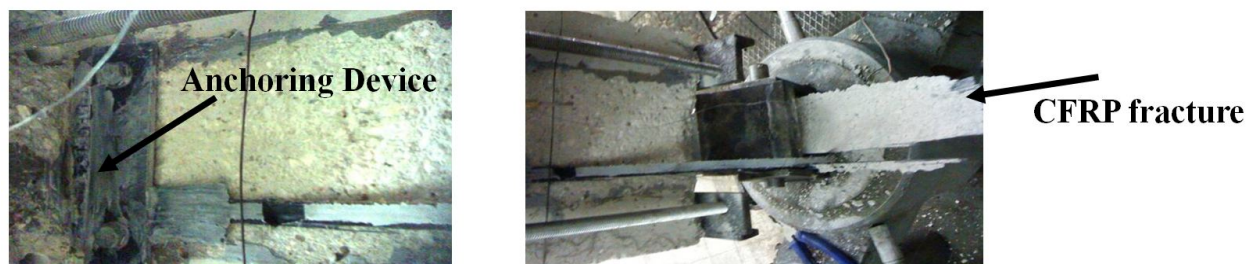
Figure 48. Detail of the anchoring device and the fracture of the CFRP strip when such an anchoring device is employed.
