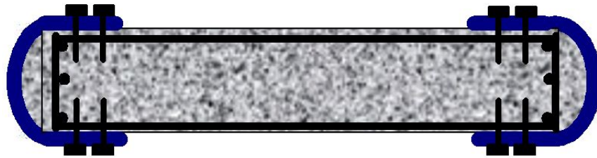
Figure 23. R/C cross-sections with one side longer than the other ( h/b > 1.5 ) and CFRP partial confinement.
