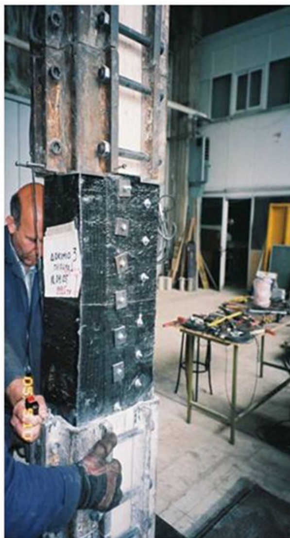
Figure 27. Specimen with confining steel brackets at the edges and partial CFRP confinement at the mid-part
