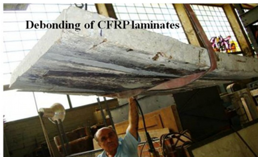
Figure 9. Flexural failure of the Ermionio slab specimen retrofitted with two CFRP laminates bonded only with epoxy paste. The CFRP laminates were debonded from the concrete slab in this case.
