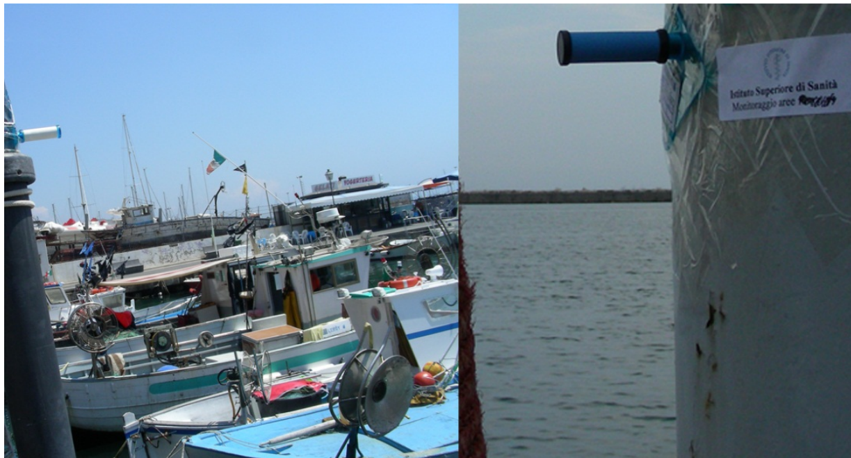
Figure 2. Two examples of VOCs monitoring in port areas using radial diffusive samplers
