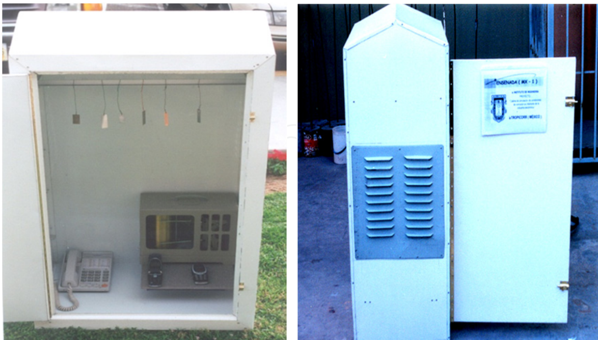
Figure 10. Simulation chamber for corrosion: left. Front view with installed specimens, Right. Side view with the ventilation device.
