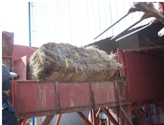
Figure 22. Thermocouples on the bale in feeding system
