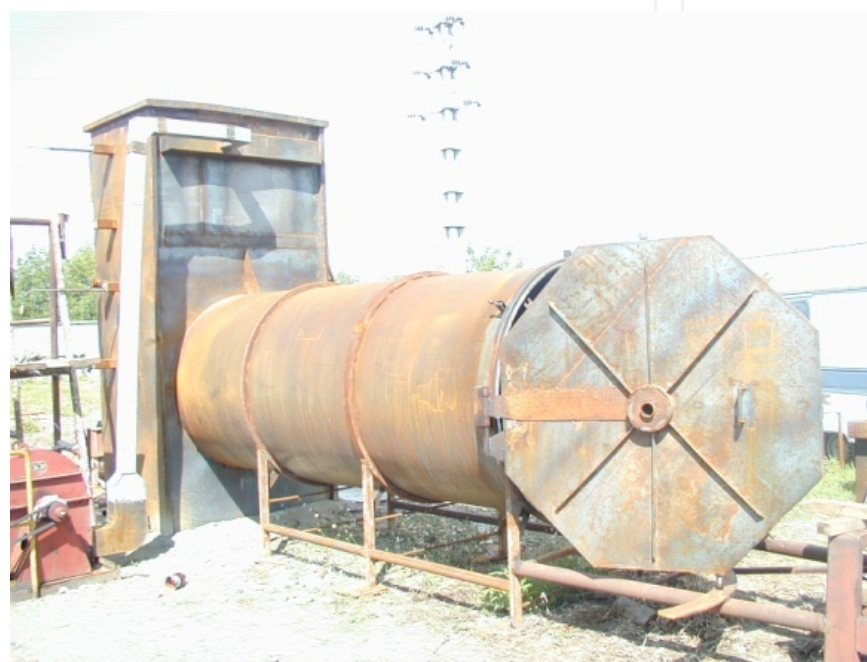
Figure 6. The appearance of the demo facility for burning large rolled straw bales
