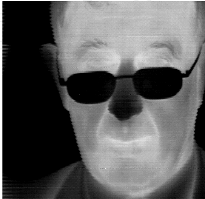
Figure 31. An example of the thermal image 288×4 PV FPA.
