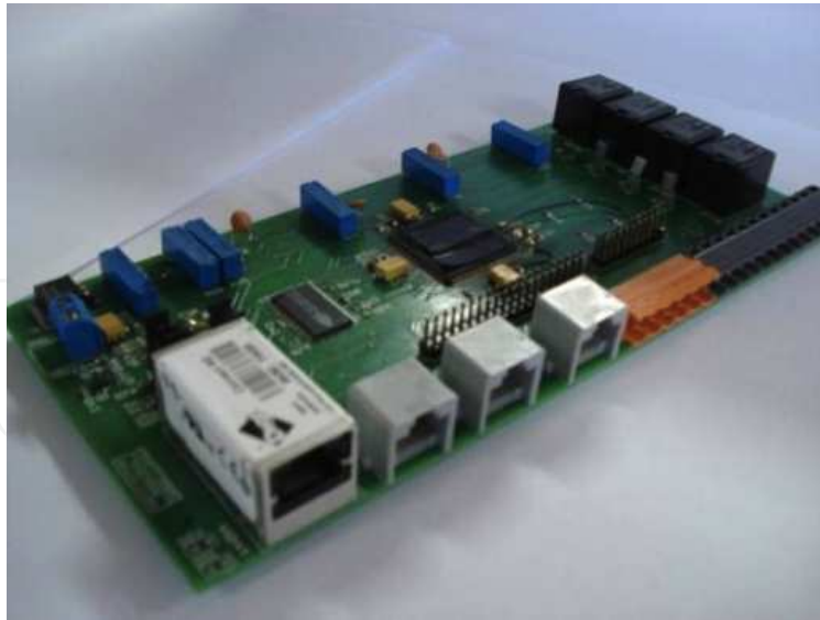
Figure 6. Remote Data Acquisition Unit - RDAU.
