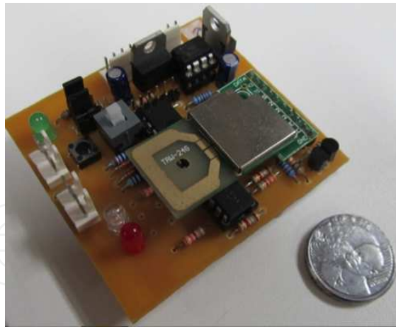
Figure 4. Intelligent Sensor Module - SSM.
