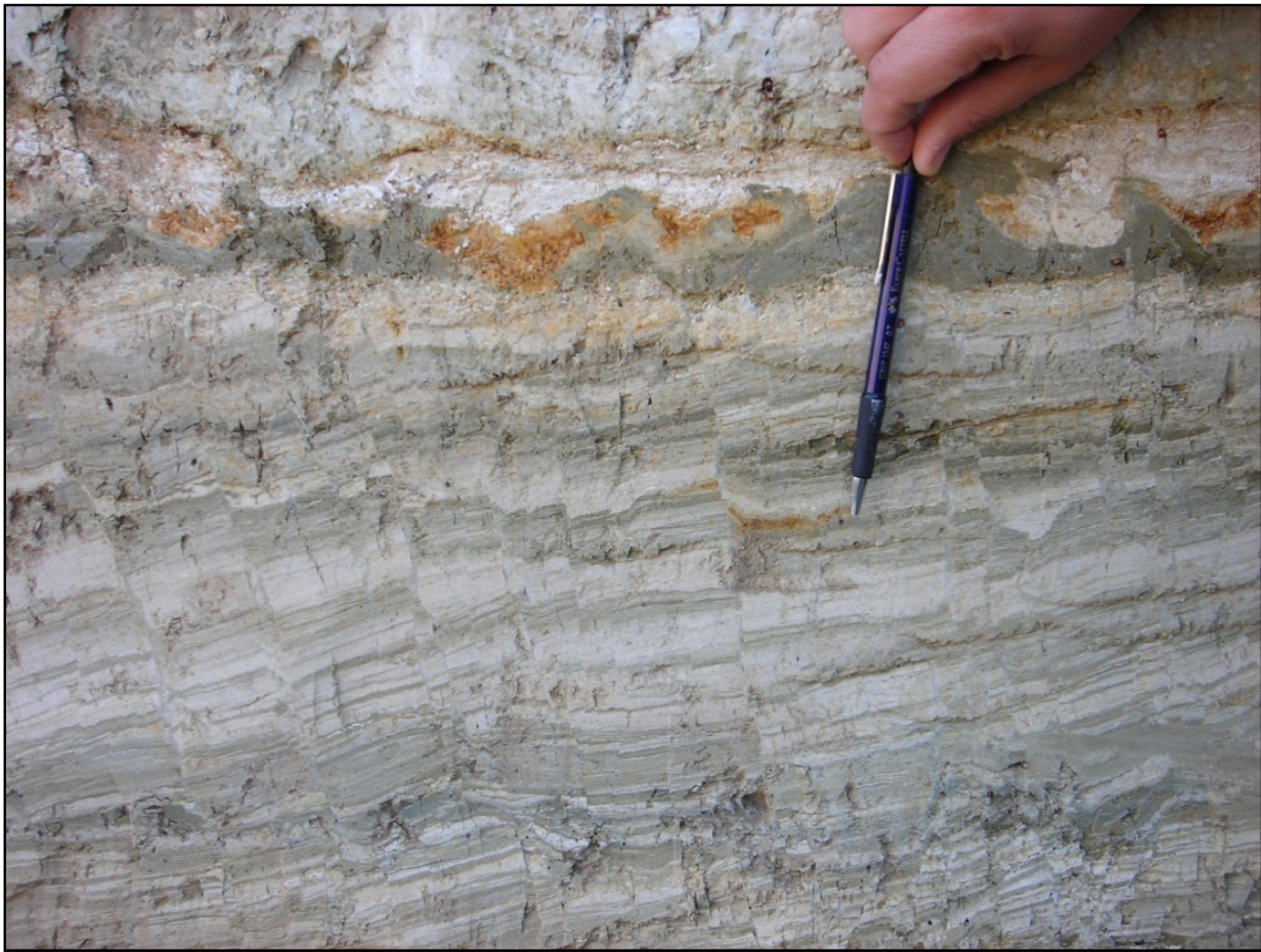
Figure 17. Small scale normal faults and paleoliquefaction structures observed between 14 th and 15 th meters of Tevfikiye Trench (Look from West to East)
