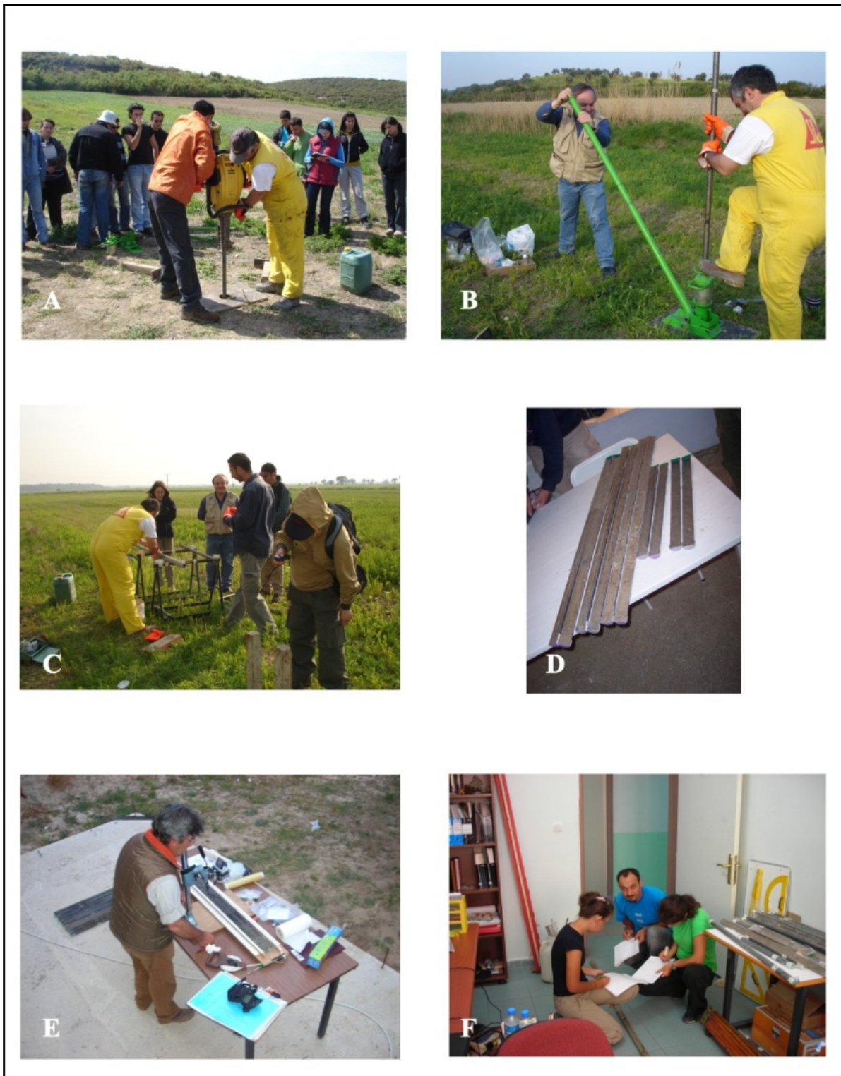
Figure 12. Phases of shallow drill works A: Drilling, B: Hoisting of drill set, C: Numeration, D: Splitting of drill cores, E: Photographing, F: Logging
