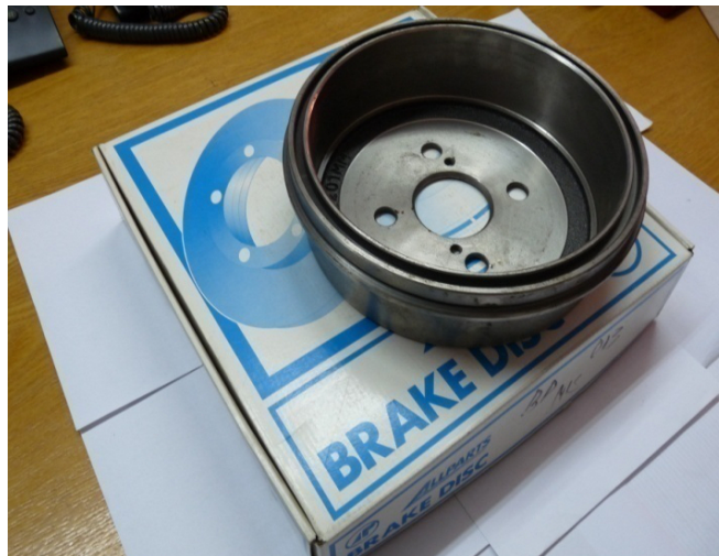
Figure 47. A Brake Drum made by PM process.
