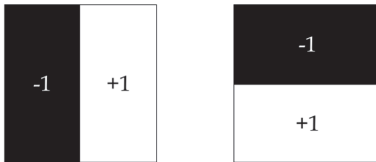
Figure 7. Haar wavelet filters to compute response for the x (left) and y (right) directions (Bay et al., 2008)
