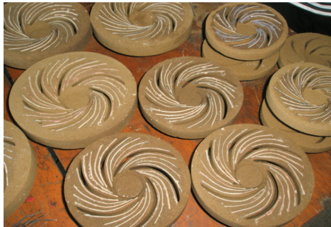
Figure 10. Examples of sand core which have rubber non-smooth structures pasted on their surface.
