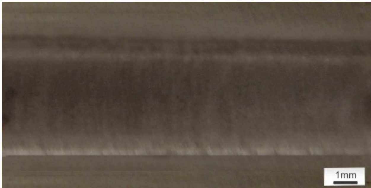
Figure 1. View of the MCMgAl9Zn1 casting magnesium alloy face of weld after laser treatment with TiC, scan rate: 0.75 m/min, laser power: 1.2 kW
