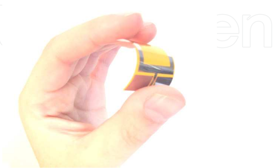
Figure 1. Flexible printed monopole antenna based on Kapton Polyimide substrate.
