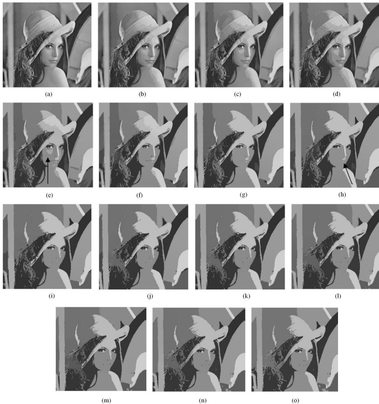
Figure 18. a) Original image (Lena), (b) Segmentation for hr = 5 and hs = 2 , 14 iterations, (c) Segmentation for hr = 7 and hs = 4 , 16 iterations, (d) Segmentation for hr = 9 and hs = 6 , 25 iterations, (e) Segmentation for hr = 11 and hs = 8 , 48 iterations, (f) Segmentation for hr = 13 and hs = 10 , 25 iterations, (g) Segmentation for hr = 15 and hs = 12 , 20 iterations, (h) Segmentation for hr = 17 and hs = 14 , 26 iterations, (i) Segmentation for hr = 19 and hs = 16 , 24 iterations, (j) Segmentation for hr = 21 and hs = 18 , 21 iterations, (k) Segmentation for hr = 23 and hs = 20 , 26 iterations, (l) Segmentation for hr = 25 and hs = 22 , 13 iterations, (m) Segmentation for hr = 27 and hs = 24 , 5 iterations, (n) Segmentation for hr = 29 and hs = 26 , 8 iterations, (o) Segmentation for hr = 31 and hs = 28 , 10 iterations. The arrows indicate the permanency of stains for those window sizes.
