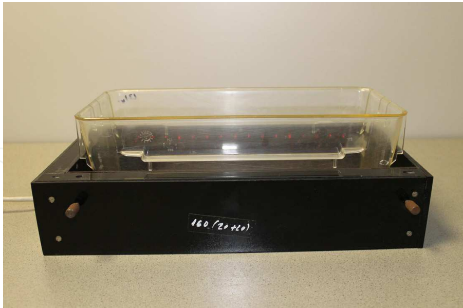
Fig. 2. Complementary tests: Actimeter. This apparatus registers the spontaneous locomotor activity of the animals by means of an infrared photocell system.
