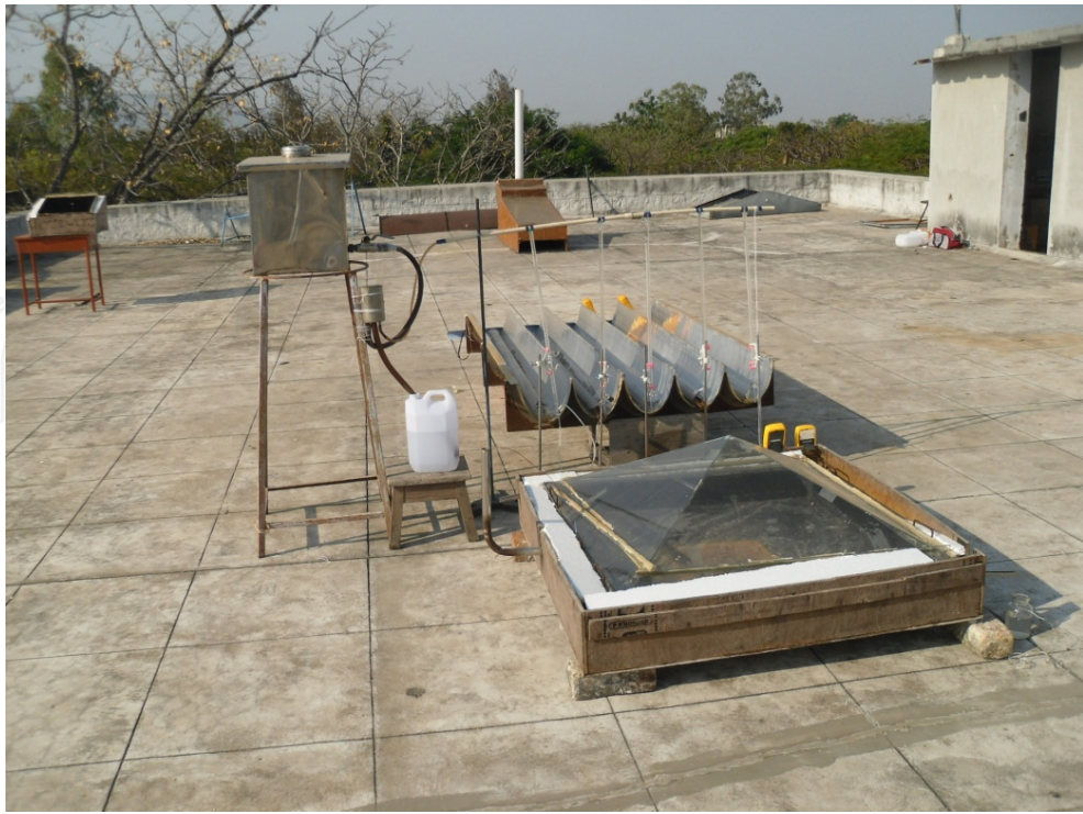
Figure 2. Pictorial view of compound parabolic concentrator tubular solar still coupled with pyramid solar still.
