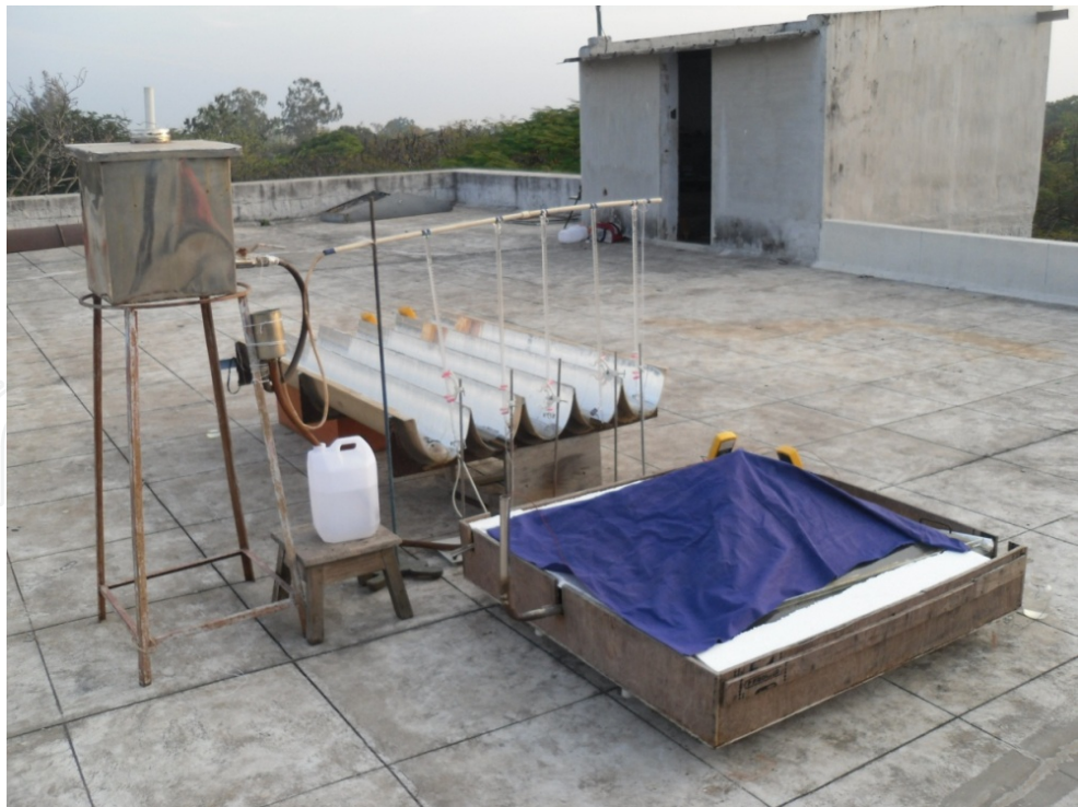
Figure 3. Pictorial view top cover closed pyramid solar still coupled with compound parabolic concentrator tubular solar still.
