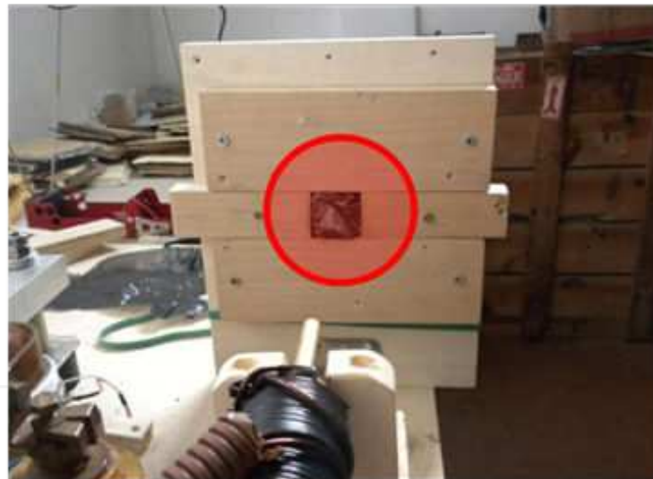
Figure 14. Picture of the plasticine witness located in the square hole of the sample's support in front of the CG barrel.
