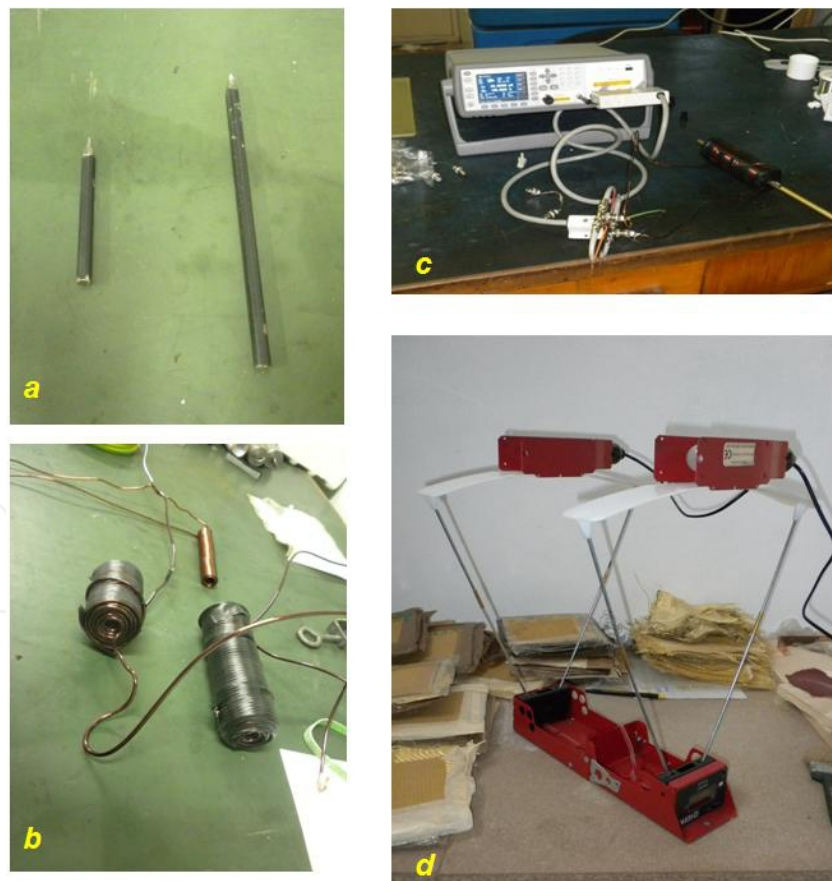
Figure 10. CG set-up pictures: a) short (S) and long (L) iron bullets; b) different copper coils tested; C) inductance static measurements by Agilent LCR Meters; d) ballistic ProChrono chronograph for bullet's speed measurements.
