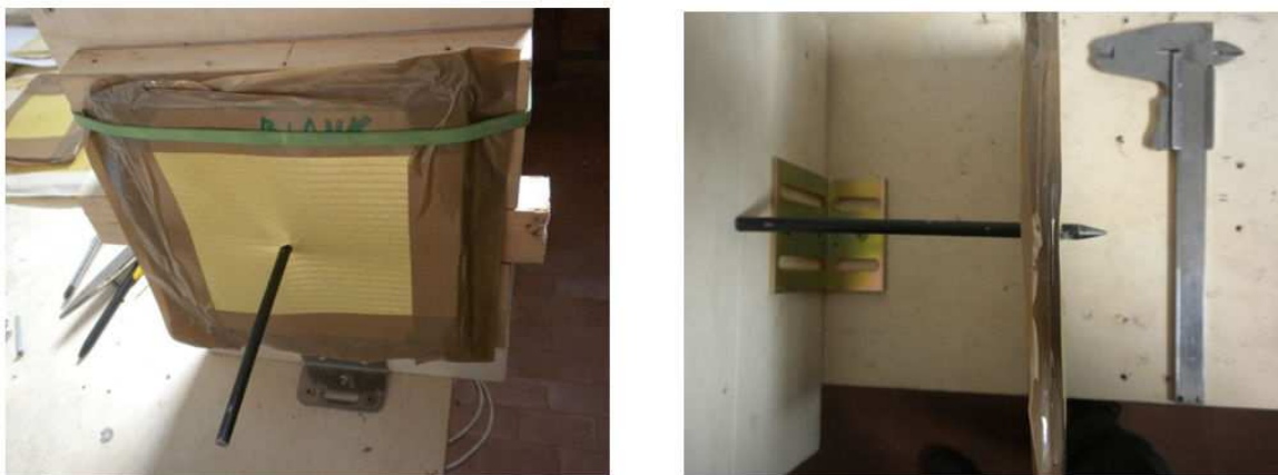
Figure 15. Pictures of a panel sample just after the ballistic test.
