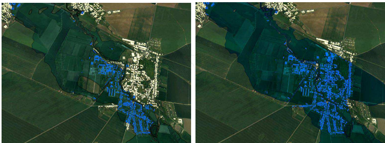
Fig. 13. Simulation of affected areas (blue) and not affected areas (white) during a flood 1994 (left); simulation with planned dams (right) (Buhmann & Pietsch, 2008a)
