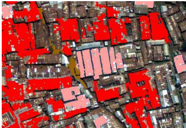
Fig. 7. Selecting training samples for supervised classification (Feature Extraction module of ENVI EX).
