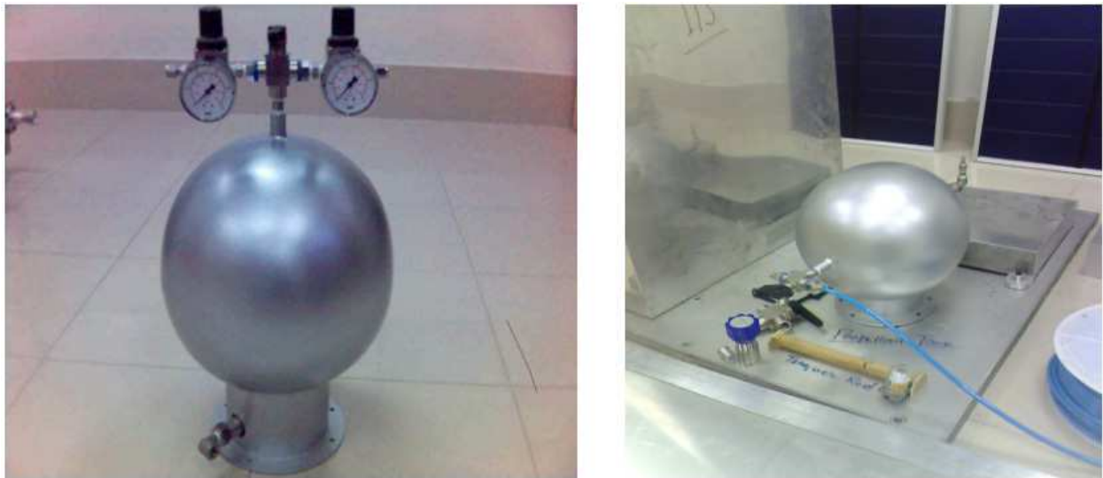
Fig. 8. Installation of Propellant Tank on PRSS Structure
