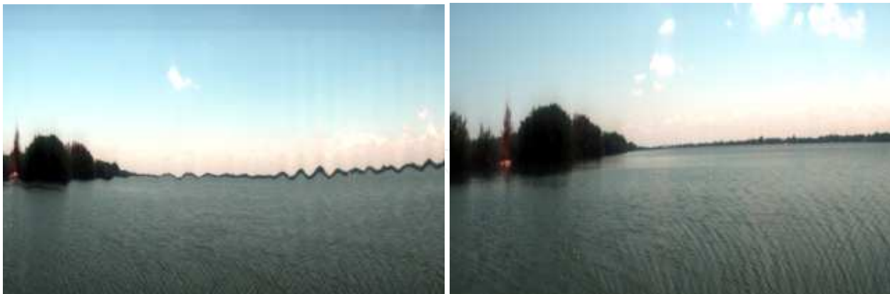
Fig. 15. A hyperspectral image (left) 3 band RGB display of a littoral zone using a pushbroom sensor mounted on a vessel anchored at two points. During the acquisition of the hyperspectral image the sensor records the pitching effect of the anchored vessel that needs to be corrected using an IMU sensor due to the water surface gravity waves. The influence of this motion can clearly be seen in the image if no correction is applied (left). The shoreline area (right) acquired when the pushbroom sensor was mounted on fixed platform above the water. In this case no correction needs to be applied to the image. Note the clarity of the water surface capillary and small gravity waves.
