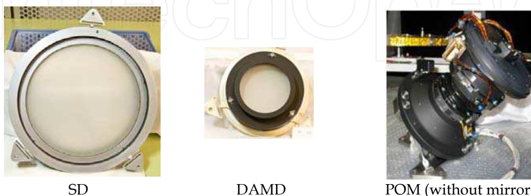
Fig. 8. On-board calibration devices SD, DAMD and pointing mirror mechanism POM
