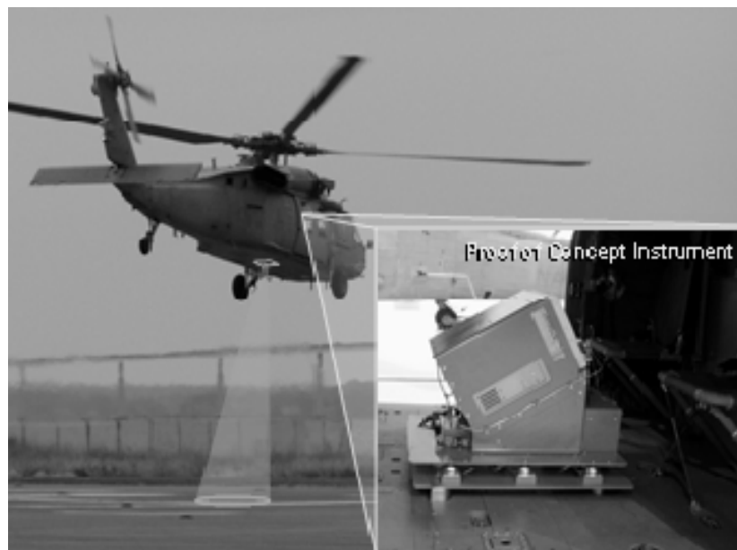
Fig. 16. DiBAR Instrument Installed in vehicle for initial flight tests.
