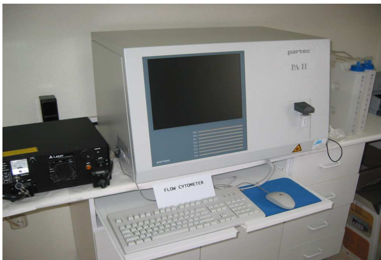
Fig. 2. Flow cytometer used for estimation of nuclear DNA content
