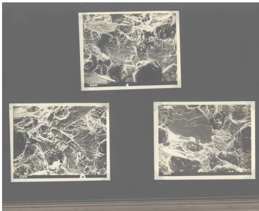
Figure 14. Transgranular cleavage in crack growth region of 3% Si casting Source: S. Seetharamu [10]
