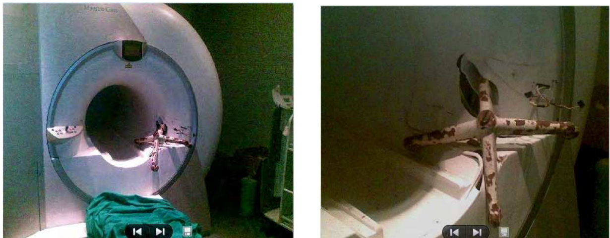
Fig. 5. Photographs of a hanger of saline physiology stucked to the MRI (Sezdi, 2009a)
