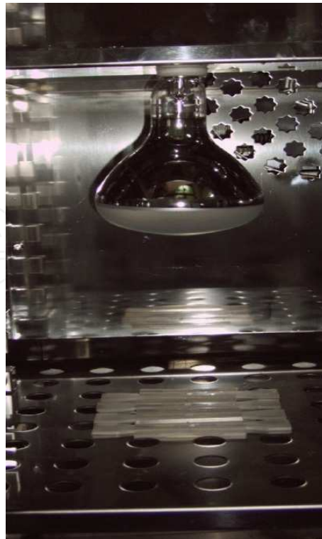
Fig. 1. Inside the climate chamber with 5 samples
