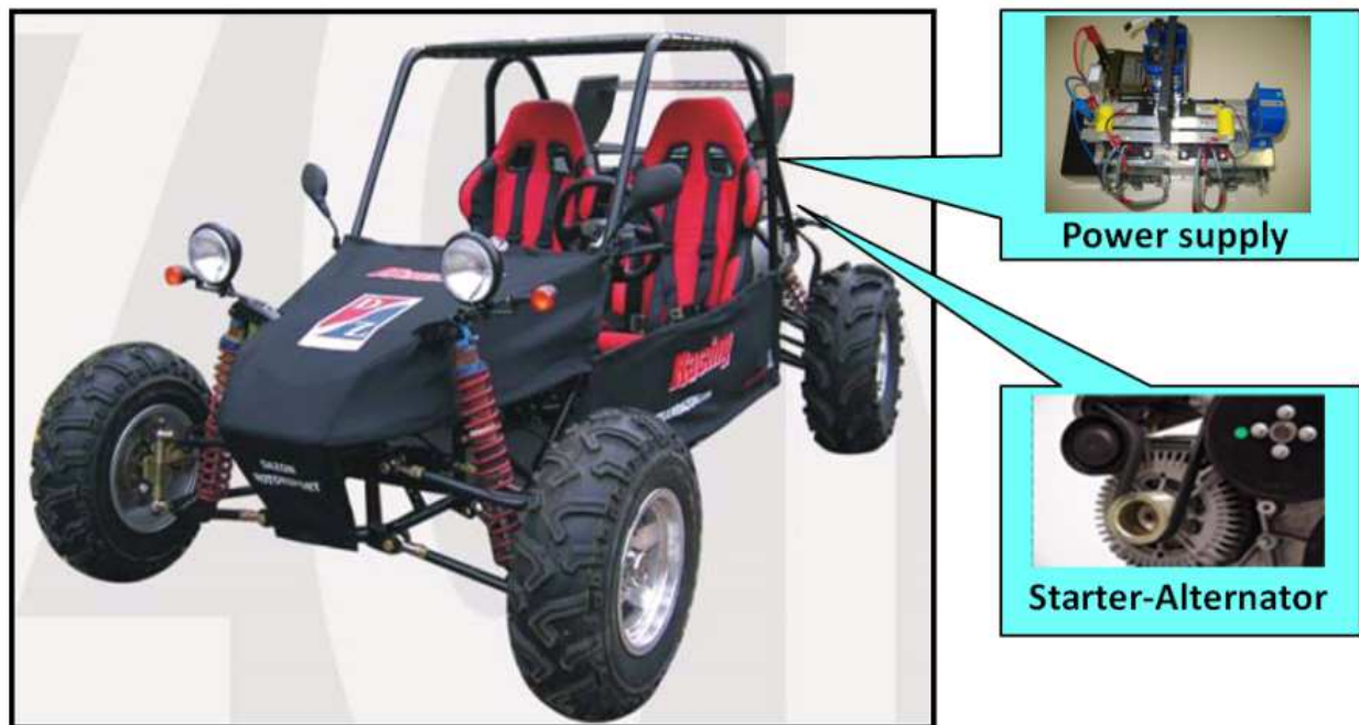
Fig. 3. Using the hybrid supply with starter or starter-alternator
