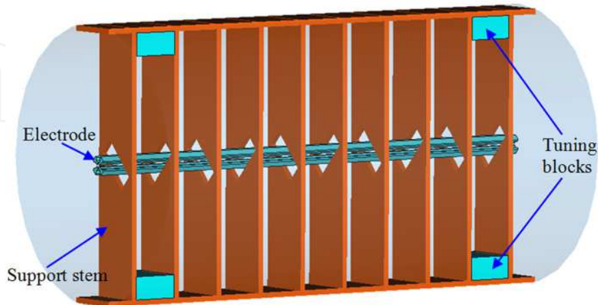
Fig. 4. MWS simulation model of the ladder IH-RFQ.
