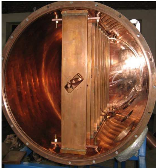
Fig. 10. The constructed ladder IH-RFQ cavity.
