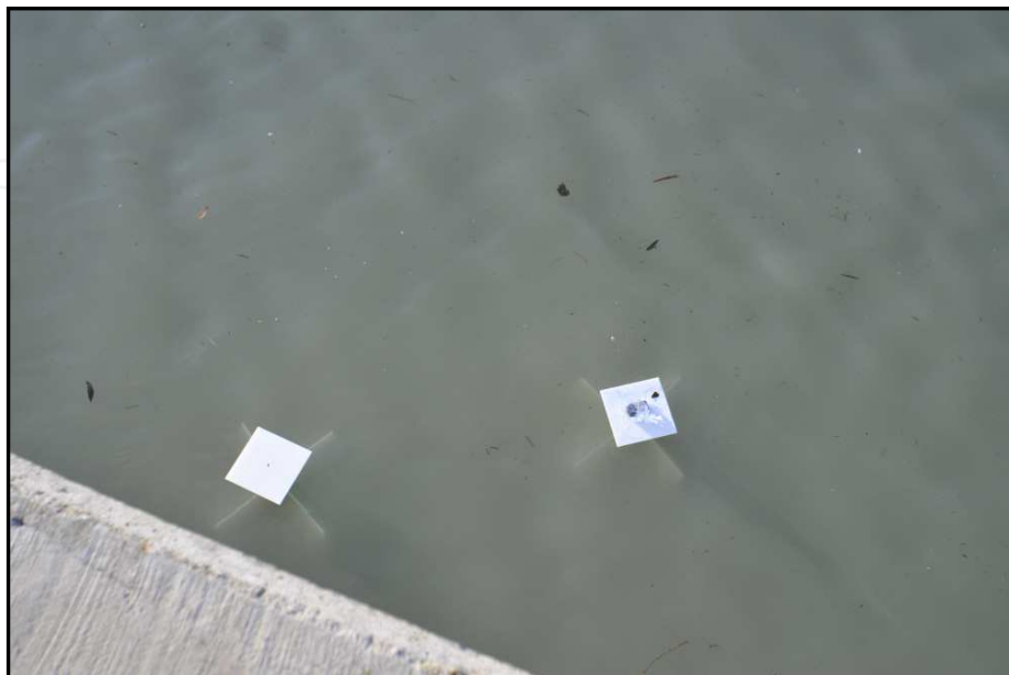
Fig. 7. Two drifting buoys during the preliminary tests.
