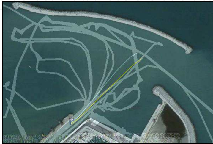
Fig. 10. Raw trajectories of the Lagrangian buoys as measured by the GPS. The white and yellow line represent the two buoys trajectories during the preliminary tests.
