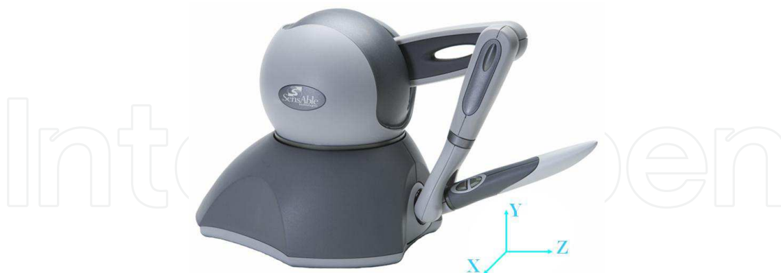
Fig. 12. Coordinate system of Phantom Omni
