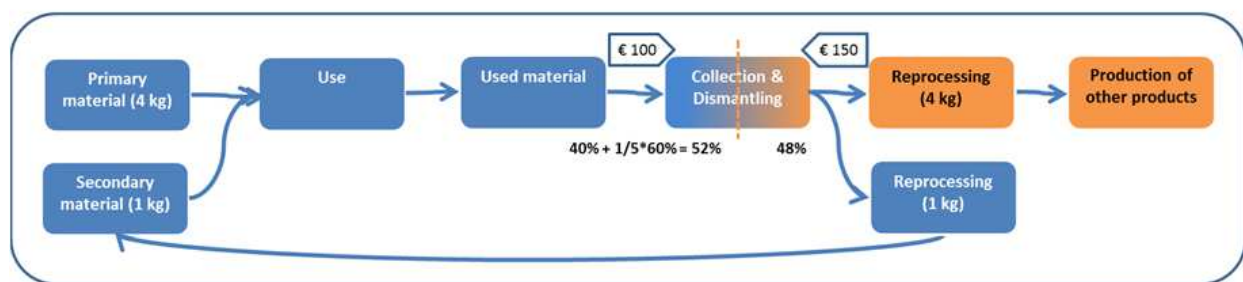
Fig. 10. Example of economic allocation of inputs and outputs of a semi-closed loop recycling system (based on Guinee et al., 2004). The used material is based on its economic value allocated 40% of the impact of the collection and dismantling.
