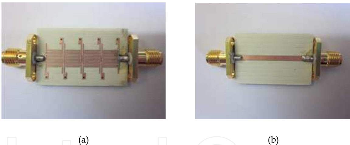
Fig. 10. Prototypes of TTDLs using (a) four CRLH TL unit cells and (b) RH TL
