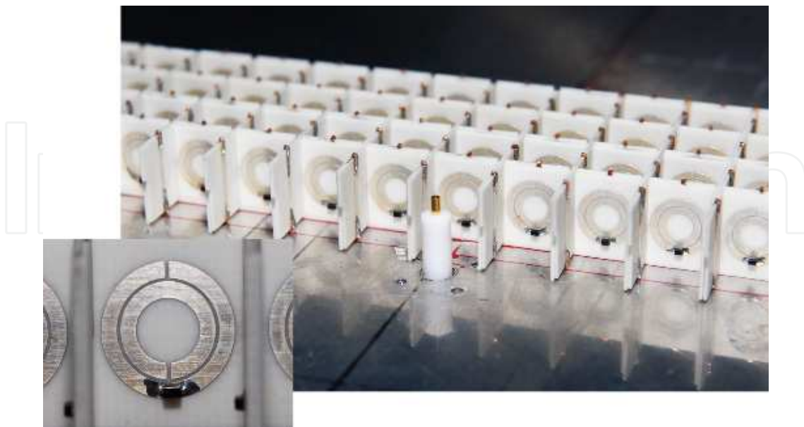
Fig. 14. Photograph of the nonlinear tunable metamaterial created by square arrays of wires and nonlinear SRRs. Each SRR contains a varactor (see the inset) which provides power-dependent nonlinear response.
