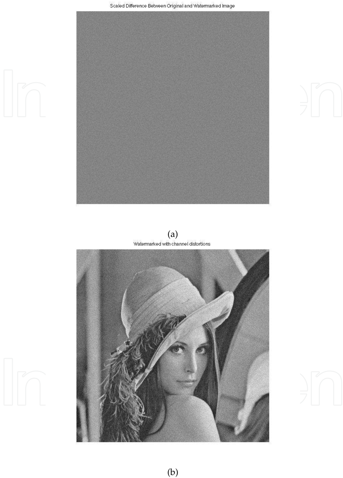
Fig. 3. (a) Difference between the original and the watermarked Image (scaled by 10 and added 128), (b) Watermarked Image attacked with AWGN noise \sim N(0,10) . Very robust to AWGN, P_{error} \leq 1E - 6 .
