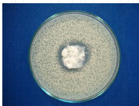
Photo 2. Growth inhibition zone around the C. albicans polypropylene fibers containing 2% Ingaguard- method according to SN 195921
