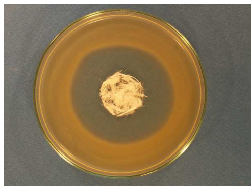
Photo 1. Growth inhibition zone around the S. aureus ; polypropylene fibers containing 2% Ingaguard- method according to SN 195 920
