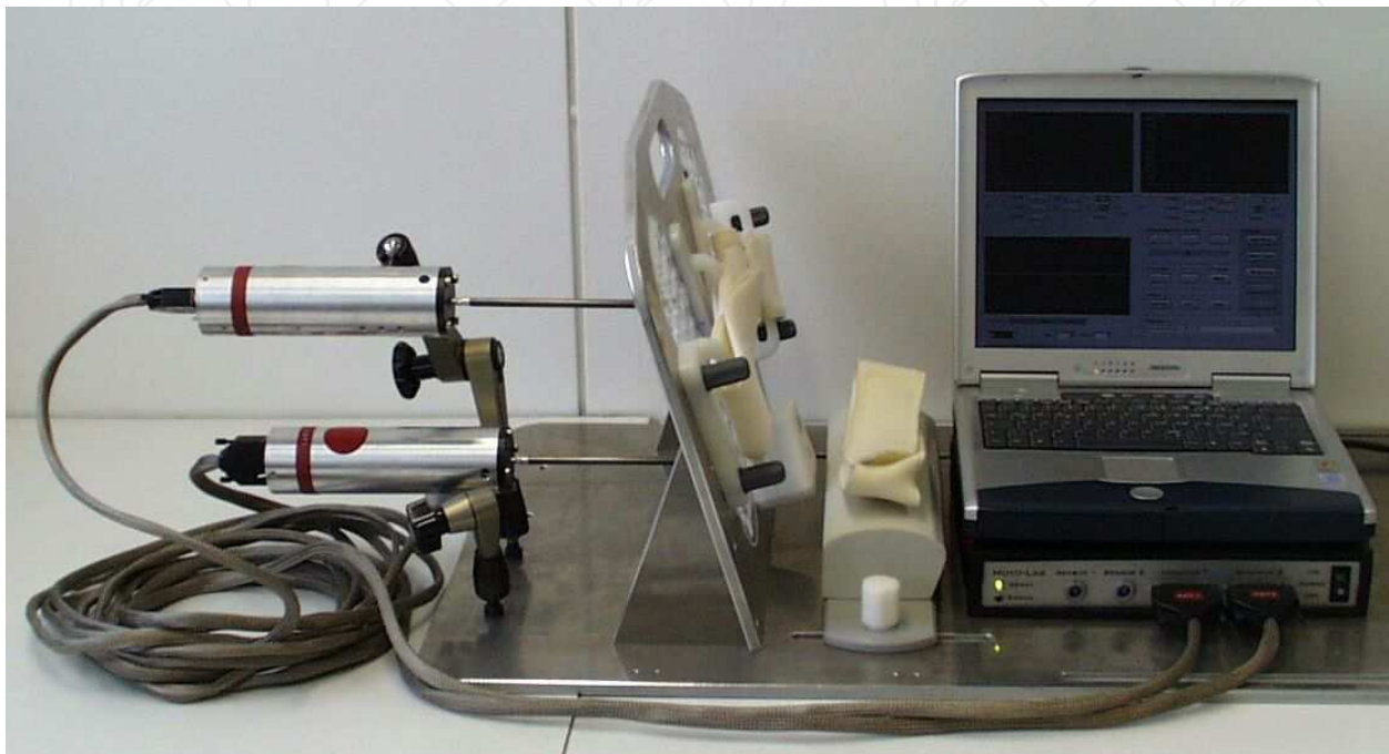
Fig. 2. Example of an electromagnetic vibrotactile stimulation system (Gallasch et al., 2006).
