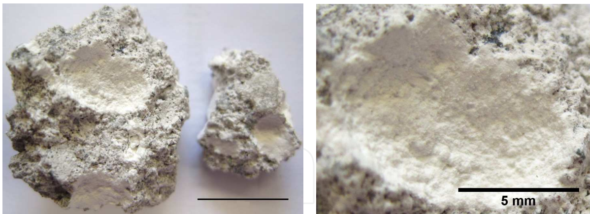
Fig. 1. Pure lime lumps in a specimen of air lime mortar (left hand side; scale bar: 1 cm) and detail of the lime lump (right hand side)
