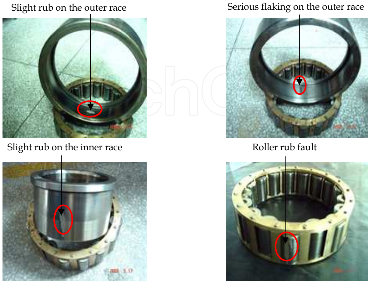
Fig. 6. Faults in the locomotive rolling bearings.
