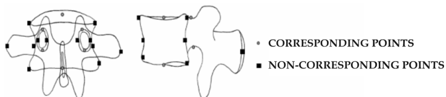
Fig. 17. Corresponding and non corresponding points on an AP and lateral radiographic shadows of a vertebra for a stereo-graphic 3D reconstruction technique.
