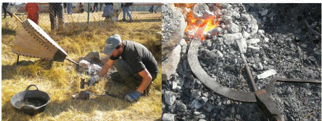
Fig. 16. Experimental process of an iron sickle forging and production
