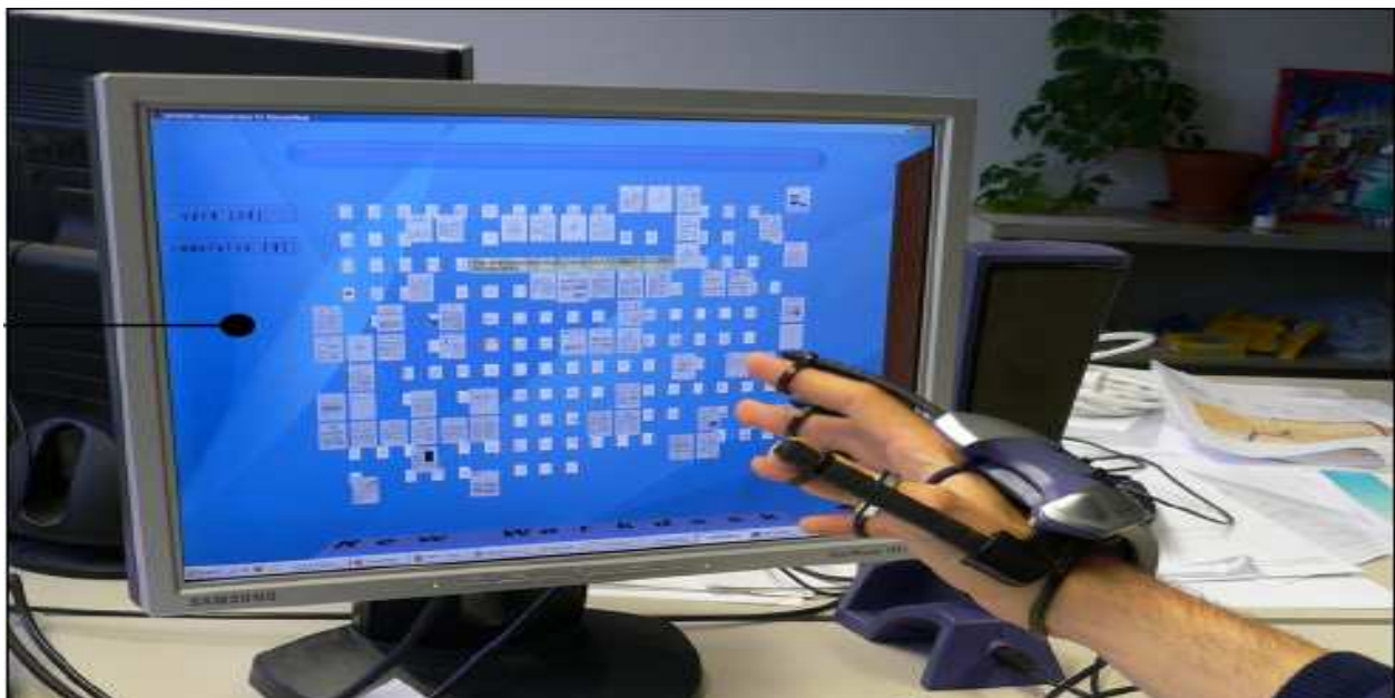
Fig. 7. Illustration of navigation through a virtual environment with data-glove (Baumgärtner et al. (2007))
