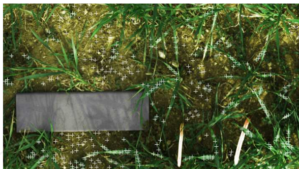
Fig. 15. Calibration image and sample positions (the reference ceramic can be seen on the left)
