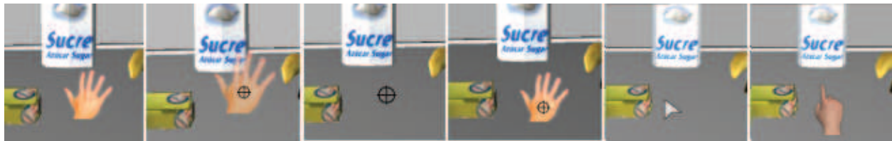
Fig. 1. The six cursors tested. From left to right: opaque hand, transparent hand + spy-hole, spy-hole, opaque hand + spy-hole, arrow, pointing finger
