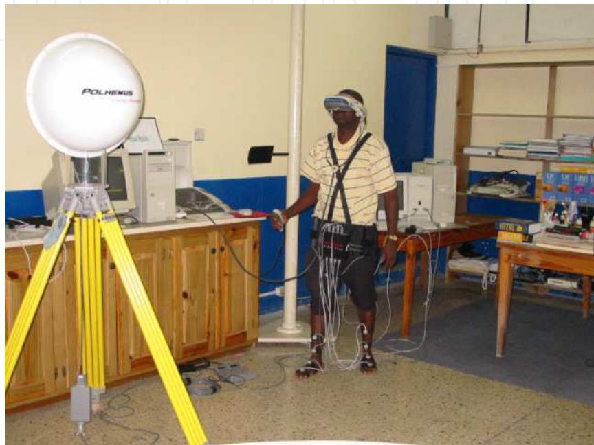
Fig. 3. The Author with the i-glasses PC 3D HR Head Mounted Display and the Polhemus electromagnetic tracker system (Akinladejo, 2005)
