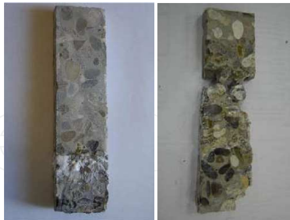
Fig. 22. Visual observation of concrete specimens partially exposed to \text{Na}_2\text{SO}_4 and \text{MgSO}_4 solutions [53]
