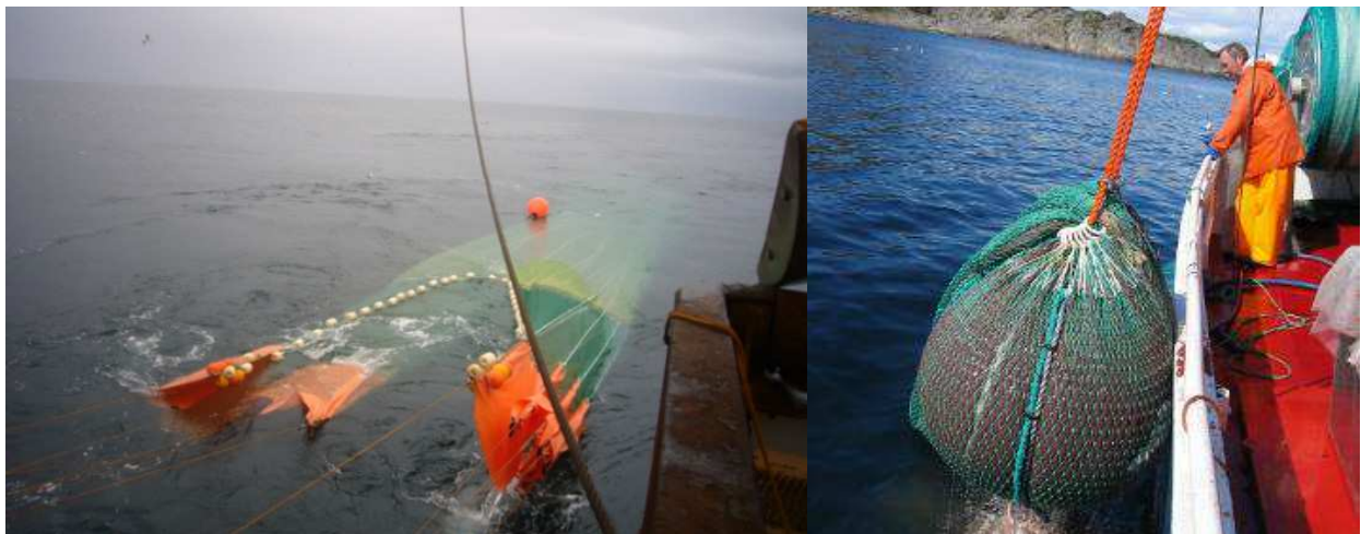
Fig. 1. Full scale test of a commercial zooplankton trawl (left), and 1200 kg of copepods ( Calanus sp.) caught after one hour tow (right). Photo: Snorre Angell, Calanus AS.
