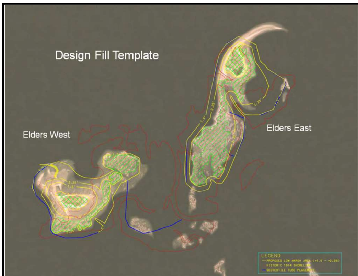
Fig. 4. Design fill template for Elders Point East and Elders Point West based on the 1974 shoreline limits.
