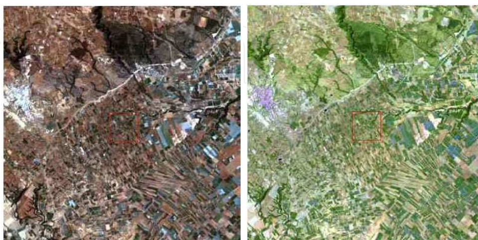
Fig. 2a. Landsat Image: True colours. Fig. 2b. Landsat Image: False colours (RGB: band 7,5,3).
